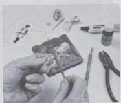
2. Trimming. Cut off the parts from the ingate with a pliers. Trim the joints and any flash and parting line. A common mistake is that the neck is not trimmed short enough. Make sure the pieces fit well together.
