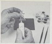
1. Stick one or more figures on a piece of hardboard with a glue pad or hobby adhesive to hold the figure while painting.
